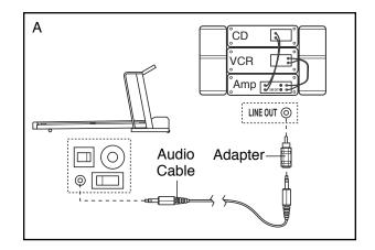
B. Plug one end of the audio cable into the jack on the front of the treadmill near the power cord. Plug the other end of the cable into the included adapter. Plug the adapter into an RCA adapter (available at electronics stores). Next, remove the wire that is currently plugged into the LINE OUT jack on your stereo and plug the wire into the unused side of the RCA adapter. Plug the RCA adapter into the LINE OUT jack on your stereo.
